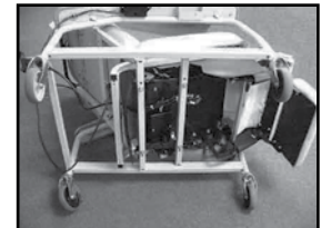
Roll Recliner onto its Left Side
