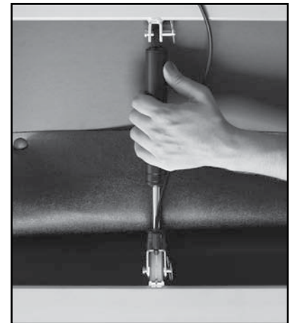
Adjusting Cable Tension 1
