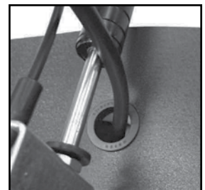
Insert Cable Connector Labeled SEAT Through Bushing
