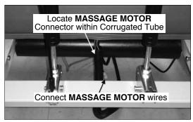
Connect Massage Motor Wires
