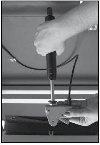
**Adjusting Cable Tension 2**
