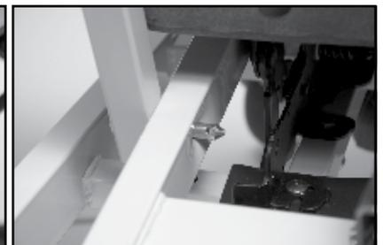
7. Secure the two clevis pins by placing a large cotter pin through the hole in the clevis pin (one for each side) as shown at right.
